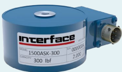
1500 Low Capacity LowProfile™ Load Cell 25 lbf to 300 lbf 111 N to 1.33 kN
