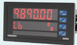
9890 Strain Gage, Load Cell, & mV/V Indicator ±15, ±25, ±150, ±250 mV Bipolar Input Ranges Powers up to 12 x 350 ohm Sensors
