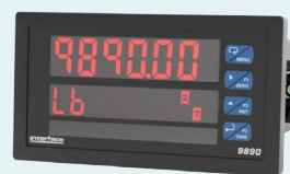
9890 Strain Gage, Load Cell, & mV/V Indicator ±15, ±25, ±150, ±250 mV Bipolar Input Ranges Powers up to 12 x 350 ohm Sensors
