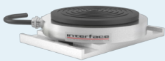
BPL Ultra Low Height Compression Only 50 lbf to 500 lbf 250 N to 2,500 N Self-Centering in all Directions High Output 4 mV/V
