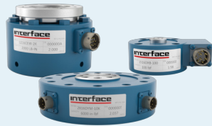
1216/1516/2816 Axial Torsion Force: 100 to 15K lbf Torque: 50 to 7.5K lbf-in Force: 1.11 to 66.7 kN Torque: 5.6 to 847 Nm Fz, Mz
